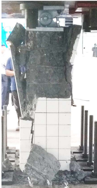
Figure 4. The failure mode of specimen CS.
